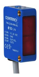
Contrinex photoelectric sensor, rectangular, polarized retroreflective, visible red light emission, 20-4200mm sensing distance, complementary light-on/dark-on, PNP, potentiometer, 4-wire, pigtail.
