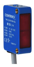
Contrinex photoelectric sensor, rectangular, polarized retroreflective, visible red, 20-4200mm sensing distance, complementary light-on/dark-on, PNP, potentiometer, 4-wire, pigtail.
