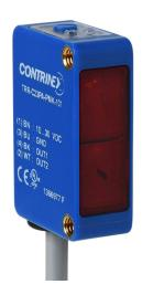
Contrinex photoelectric sensor, rectangular, polarized retroreflective, visible red, 20-4200mm sensing distance, complementary light-on/dark-on, NPN, potentiometer, 4-wire, pigtail.
