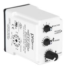
ProSense multi-mode relay timer, 0.05 seconds to 100 hours selectable timing range, 24-240 VAC and 12-125 VDC operating voltage, 10A contact rating, (1) DPDT timed relay output(s), socket mount, 11-pin. Requires Macromatic 70170-D relay socket.
