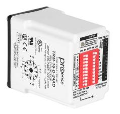
ProSense multi-mode relay timer, 0.05 seconds to 10,230 hours selectable timing range, 24 VAC/VDC operating voltage, 10A contact rating, (1) DPDT timed relay output(s), socket mount, 11-pin. Requires Macromatic 70170-D relay socket.
