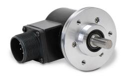
Koyo TRDA-25 series incremental (quadrature) rotary encoder, medium duty, 5 VDC, radial exit, line driver (differential) output, 500 ppr, 3/8in solid shaft, flange mount, 2in diameter body, IP65, 10-pin Military Style (MS) connector.
