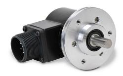
Koyo TRDA-25 series incremental (quadrature) rotary encoder, medium duty, 5 VDC, radial exit, line driver (differential) output, 360 ppr, 3/8in solid shaft, flange mount, 2in diameter body, IP65, 10-pin Military Style (MS) connector.
