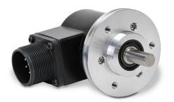
Koyo TRDA-25 series incremental (quadrature) rotary encoder, medium duty, 5 VDC, radial exit, line driver (differential) output, 2500 ppr, 3/8in solid shaft, flange mount, 2in diameter body, IP65, 10-pin Military Style (MS) connector.
