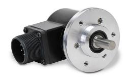
Koyo TRDA-25 series incremental (quadrature) rotary encoder, medium duty, 5 VDC, radial exit, line driver (differential) output, 1024 ppr, 3/8in solid shaft, flange mount, 2in diameter body, IP65, 10-pin Military Style (MS) connector.
