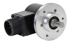
Koyo TRDA-25 series incremental (quadrature) rotary encoder, medium duty, 5 VDC, radial exit, line driver (differential) output, 100 ppr, 3/8in solid shaft, flange mount, 2in diameter body, IP65, 10-pin Military Style (MS) connector.
