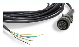
AutomationDirect encoder cable, 7-pin Military Style (MS) to pigtail, 30ft cable length. For use with Koyo TRDA-25N series encoders with push-pull (totem) output.
