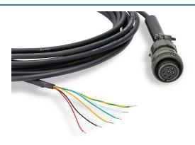
AutomationDirect encoder cable, 7-pin Military Style (MS) to pigtail, 20ft cable length. For use with Koyo TRDA-25N series encoders with push-pull (totem) output.
