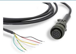
AutomationDirect encoder cable, 7-pin Military Style (MS) to pigtail, 10ft cable length. For use with Koyo TRDA-25N series encoders with push-pull (totem) output.
