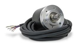
Koyo TRDA-20 series incremental (quadrature) rotary encoder, medium duty, 5 VDC, radial exit, line driver (differential) output, 360 ppr, 3/8in solid shaft, 2in diameter body, IP50, 6.5ft/2m cable length, pigtail.
