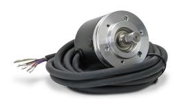
Koyo TRDA-20 series incremental (quadrature) rotary encoder, medium duty, 5 VDC, radial exit, line driver (differential) output, 1024 ppr, 3/8in solid shaft, 2in diameter body, IP50, 6.5ft/2m cable length, pigtail.
