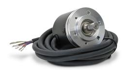
Koyo TRDA-20 series incremental (quadrature) rotary encoder, medium duty, 5 VDC, radial exit, line driver (differential) output, 100 ppr, 3/8in solid shaft, 2in diameter body, IP50, 6.5ft/2m cable length, pigtail.
