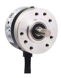
Koyo TRD-SR series incremental (quadrature) rotary encoder, light duty, 5 VDC, radial exit, line driver (differential) output, 1024 ppr, 6mm solid shaft, 38mm diameter body, IP50, 6.5ft/2m cable length, pigtail.
