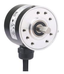
Koyo TRD-SR series incremental (quadrature) rotary encoder, light duty, 5 VDC, radial exit, line driver (differential) output, 100 ppr, 6mm solid shaft, 40mm diameter body, IP65, 6.5ft/2m cable length, pigtail.
