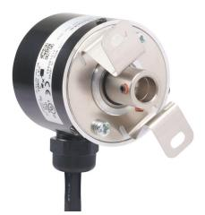
Koyo TRD-SR series incremental (quadrature) rotary encoder, light duty, 5-26 VDC, radial exit, NPN open collector output, 500 ppr, 8mm hollow shaft, 40mm diameter body, IP65, 6.5ft/2m cable length, pigtail.
