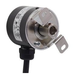
Koyo TRD-SR series incremental (quadrature) rotary encoder, light duty, 5 VDC, radial exit, line driver (differential) output, 360 ppr, 8mm hollow shaft, 40mm diameter body, IP65, 6.5ft/2m cable length, pigtail.
