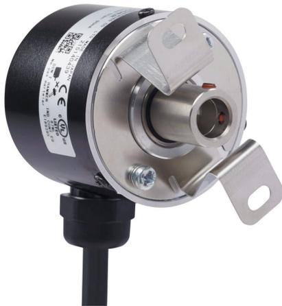
Koyo TRD-SR series incremental (quadrature) rotary encoder, light duty, 5-26 VDC, radial exit, NPN open collector output, 360 ppr, 8mm hollow shaft, 40mm diameter body, IP65, 6.5ft/2m cable length, pigtail.
