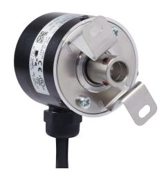
Koyo TRD-SR series incremental (quadrature) rotary encoder, light duty, 5 VDC, radial exit, line driver (differential) output, 200 ppr, 8mm hollow shaft, 40mm diameter body, IP65, 6.5ft/2m cable length, pigtail.
