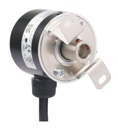
Koyo TRD-SR series incremental (quadrature) rotary encoder, light duty, 5-26 VDC, radial exit, NPN open collector output, 200 ppr, 8mm hollow shaft, 40mm diameter body, IP65, 6.5ft/2m cable length, pigtail.
