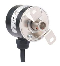
Koyo TRD-SR series incremental (quadrature) rotary encoder, light duty, 5 VDC, radial exit, line driver (differential) output, 2000 ppr, 8mm hollow shaft, 40mm diameter body, IP65, 6.5ft/2m cable length, pigtail.
