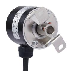
Koyo TRD-SR series incremental (quadrature) rotary encoder, light duty, 5 VDC, radial exit, line driver (differential) output, 100 ppr, 8mm hollow shaft, 40mm diameter body, IP65, 6.5ft/2m cable length, pigtail.
