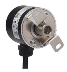
Koyo TRD-SR series incremental (quadrature) rotary encoder, light duty, 5-26 VDC, radial exit, NPN open collector output, 100 ppr, 8mm hollow shaft, 40mm diameter body, IP65, 6.5ft/2m cable length, pigtail.
