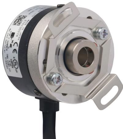
Koyo TRD-SR series incremental (quadrature) rotary encoder, light duty, 5 VDC, radial exit, line driver (differential) output, 1000 ppr, 8mm hollow shaft, 38mm diameter body, IP50, 6.5ft/2m cable length, pigtail.
