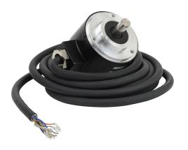
Koyo TRD-N series incremental (quadrature) rotary encoder, medium duty, 5 VDC, radial exit, line driver (differential) output, 60 ppr, 8mm solid shaft, 50mm diameter body, IP65, 6.5ft/2m cable length, pigtail.
