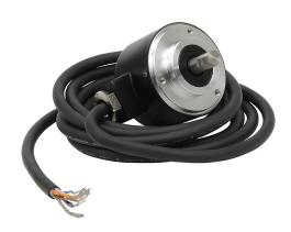
Koyo TRD-N series incremental (quadrature) rotary encoder, medium duty, 5 VDC, radial exit, line driver (differential) output, 250 ppr, 8mm solid shaft, 50mm diameter body, IP65, 6.5ft/2m cable length, pigtail.
