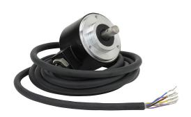
Koyo TRD-N series incremental (quadrature) rotary encoder, medium duty, 5 VDC, radial exit, line driver (differential) output, 200 ppr, 8mm solid shaft, 50mm diameter body, IP65, 6.5ft/2m cable length, pigtail.
