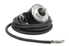
Koyo TRD-N series incremental (quadrature) rotary encoder, medium duty, 5 VDC, radial exit, line driver (differential) output, 1200 ppr, 8mm solid shaft, 50mm diameter body, IP65, 6.5ft/2m cable length, pigtail.
