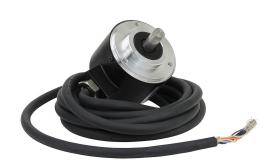
Koyo TRD-N series incremental (quadrature) rotary encoder, medium duty, 5 VDC, radial exit, line driver (differential) output, 120 ppr, 8mm solid shaft, 50mm diameter body, IP65, 6.5ft/2m cable length, pigtail.
