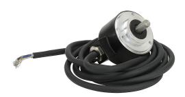
Koyo TRD-N series incremental (quadrature) rotary encoder, medium duty, 5 VDC, radial exit, line driver (differential) output, 1024 ppr, 8mm solid shaft, 50mm diameter body, IP65, 6.5ft/2m cable length, pigtail.
