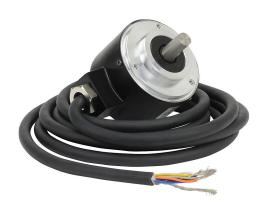
Koyo TRD-N series incremental (quadrature) rotary encoder, medium duty, 5 VDC, radial exit, line driver (differential) output, 10 ppr, 8mm solid shaft, 50mm diameter body, IP65, 6.5ft/2m cable length, pigtail.
