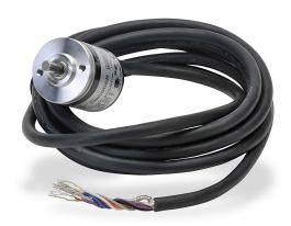
Koyo TRD-MX series incremental (quadrature) rotary encoder, light duty, 5 VDC, axial exit, line driver (differential) output, 500 ppr, 4mm solid shaft, 1in diameter body, IP50, 6.5ft/2m cable length, pigtail.
