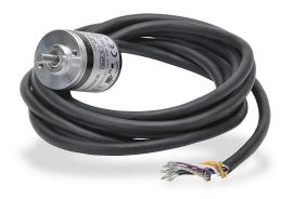
Koyo TRD-MX series incremental (quadrature) rotary encoder, light duty, 5 VDC, axial exit, line driver (differential) output, 360 ppr, 4mm solid shaft, 1in diameter body, IP50, 6.5ft/2m cable length, pigtail.
