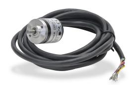
Koyo TRD-MX series incremental (quadrature) rotary encoder, light duty, 5 VDC, axial exit, line driver (differential) output, 100 ppr, 4mm solid shaft, 1in diameter body, IP50, 6.5ft/2m cable length, pigtail.
