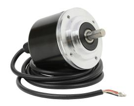
Koyo TRD-GK series incremental (quadrature) rotary encoder, heavy duty, 10-30 VDC, axial exit, push-pull (totem) output, 5000 ppr, 10mm solid shaft, 78mm diameter body, IP65, 6.5ft/2m cable length, pigtail.
