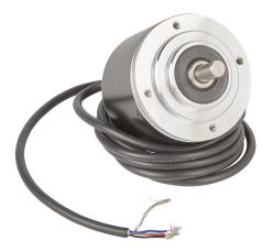
Koyo TRD-GK series incremental (quadrature) rotary encoder, heavy duty, 10-30 VDC, axial exit, push-pull (totem) output, 250 ppr, 10mm solid shaft, 78mm diameter body, IP65, 6.5ft/2m cable length, pigtail.
