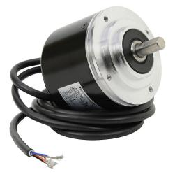
JTEKT TRD-GK series incremental (quadrature) rotary encoder, heavy duty, 10-30 VDC, axial exit, push-pull (totem) output, 1800 ppr, 10mm solid shaft, 78mm diameter body, IP65, 6.5ft/2m cable length, pigtail.
