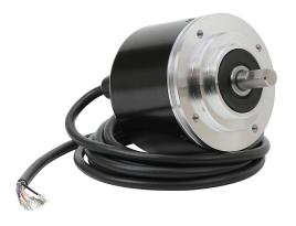
Koyo TRD-GK series incremental (quadrature) rotary encoder, heavy duty, 10-30 VDC, axial exit, push-pull (totem) output, 1200 ppr, 10mm solid shaft, 78mm diameter body, IP65, 6.5ft/2m cable length, pigtail.
