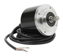
Koyo TRD-GK series incremental (quadrature) rotary encoder, heavy duty, 10-30 VDC, axial exit, push-pull (totem) output, 120 ppr, 10mm solid shaft, 78mm diameter body, IP65, 6.5ft/2m cable length, pigtail.
