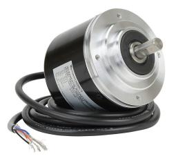
Koyo TRD-GK series incremental (quadrature) rotary encoder, heavy duty, 10-30 VDC, axial exit, push-pull (totem) output, 1000 ppr, 10mm solid shaft, 78mm diameter body, IP65, 6.5ft/2m cable length, pigtail.
