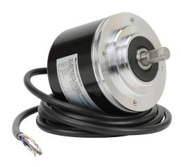
Koyo TRD-GK series incremental (quadrature) rotary encoder, heavy duty, 10-30 VDC, axial exit, push-pull (totem) output, 100 ppr, 10mm solid shaft, 78mm diameter body, IP65, 6.5ft/2m cable length, pigtail.
