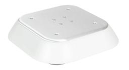
Fandis Virdis series exhaust fan, top mount, 338 CFM, 230 VAC operating voltage, NEMA 12, indoor use only, 6.89 x 6.89in enclosure cutout, RAL 7035 light gray.
