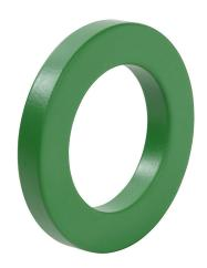
Roxburgh toroid, EMI/RFI filtering, 66mm inside diameter, 102mm outside diameter, 15mm thick. For use with all AC drives.
