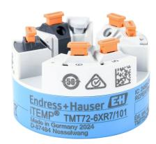
Endress+Hauser iTEMP programmable temperature transmitter, isolated, Input: 1-channel, RTD/thermocouple/bipolar voltage/potentiometer, deg F or deg C, Output: 1-channel, current/HART, 10-36 VDC operating voltage, DIN Form B connection head mount, push-in terminals.
