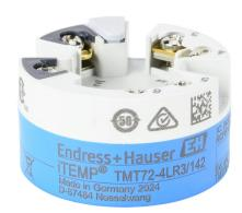
Endress+Hauser iTEMP programmable temperature transmitter, isolated, Input: 1-channel, RTD/thermocouple/bipolar voltage/potentiometer, deg F or deg C, Output: 1-channel, current/HART, 10-36 VDC operating voltage, DIN Form B connection head mount, screw terminals.
