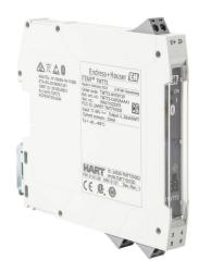
Endress+Hauser iTEMP programmable temperature transmitter, isolated, Input: 1-channel, RTD/thermocouple/bipolar voltage/potentiometer, deg F or deg C, Output: 1-channel, current/HART, 11-36 VDC operating voltage, 35mm DIN rail mount, screw terminals.
