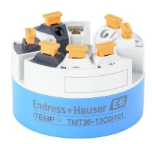
Endress+Hauser iTEMP programmable temperature transmitter, non-isolated, Input: 1-channel, RTD, deg F or deg C, Output: 1-channel, IO-Link, 18-30 VDC operating voltage, DIN Form B connection head mount, push-in terminals.
