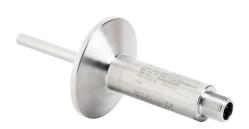
Endress+Hauser iTHERM temperature sensor/transmitter, Pt100 RTD, M12 probe, 0–150 °C, 50 mm insertion length, 6 mm probe diameter, 1-1/2 in sanitary tri-clamp process connection, Output: 1-channel, current/IO-Link, 4-pin M12 quick-disconnect.
